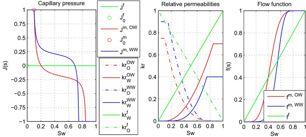
**FIGURE 1.** Relative permeability, capillary pressure and flow functions for matrix and fracture. 2 wetting states are considered for the matrix (oil-wet and water-wet). Green curves represent fracture, while red and blue curves correspond to oil-wet or water-wet matrix, respectively.
