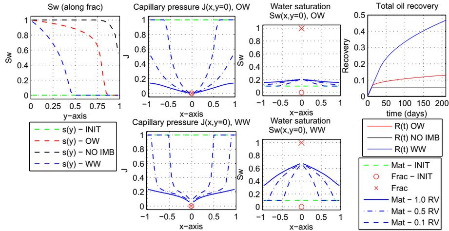
**FIGURE 2.** Water saturation along fracture (left) after injecting 1 FV water shows front delay due to imbibition. Matrix profiles at  $y = 0$  of capillary pressure  $J$  and water saturation after injecting 0.1, 0.5 and 1.0 RV of water (middle). Oil recovery profile (right) for injecting 1RV=210d shows that recovery by imbibition depends strongly on wettability.
