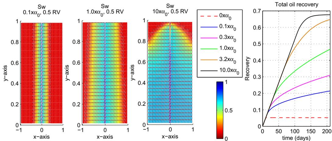
**FIGURE 3.** Impact of  $\alpha$ . Distributions of water saturation (left) and recovery profile (right). If  $\alpha$  is high imbibition dominates over fracture flow and the water effectively displaces oil. For low  $\alpha$  most of the water flows through the fracture without entering the matrix.
