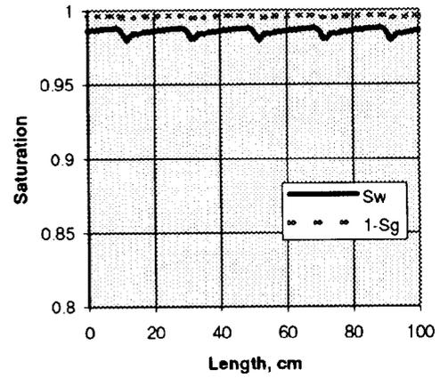
Fig. 10. Water injection at periodic boundary conditions, water wet rock
