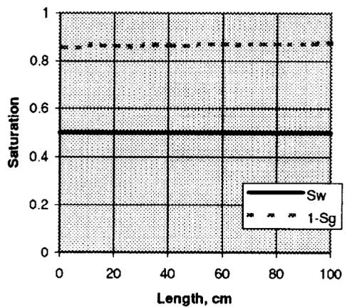
Fig. 5. Gas injection at zero capillary pressure at the outlet end, mixed-wet rock
