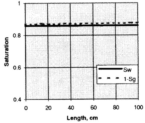
Fig. 9. Gas injection at zero capillary pressure at the outlet end, water wet rock
