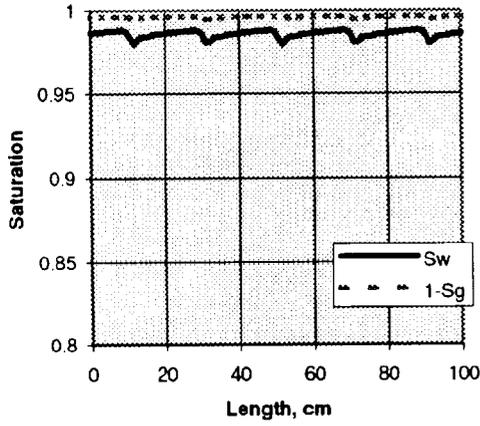
Fig. 6. Water injection at periodic boundary conditions, mixed-wet rock
