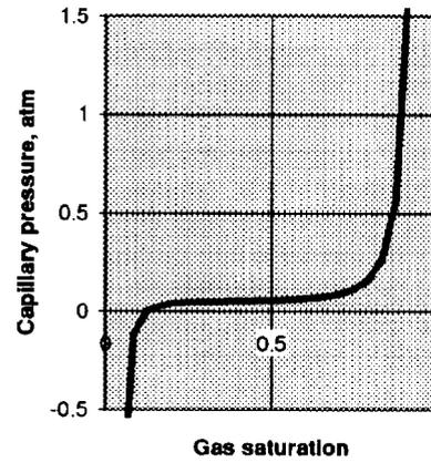
Fig. 3. Gas - oil capillary pressure corresponding to the absolute permeability 1 D.
