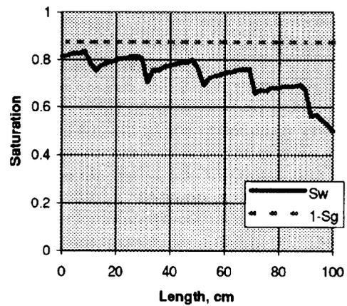
Fig. 4. Water injection at zero capillary pressure at the outlet end, mixed-wet rock
