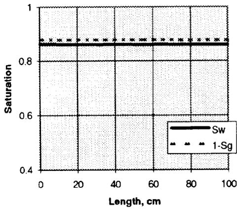
Fig. 8. Water injection at zero capillary pressure at the outlet end, water wet rock
