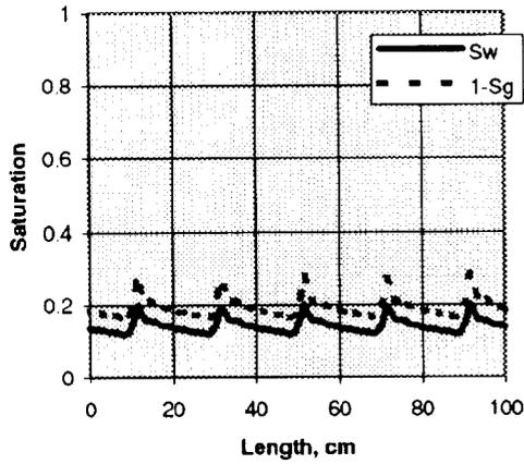
Fig. 7. Gas injection at periodic boundary conditions, mixed-wet rock
