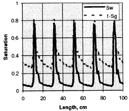
Fig. 11. Gas injection at periodic boundary conditions, water wet rock
