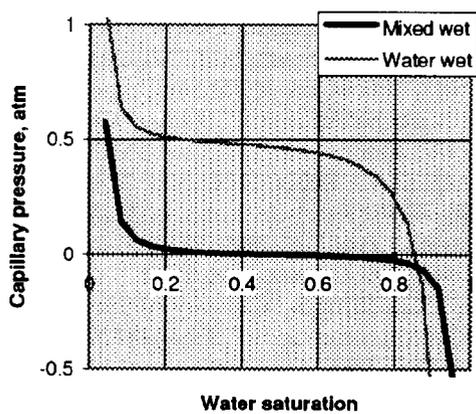
Fig. 2. Oil water capillary pressures corresponding to the absolute permeability 1 D.
