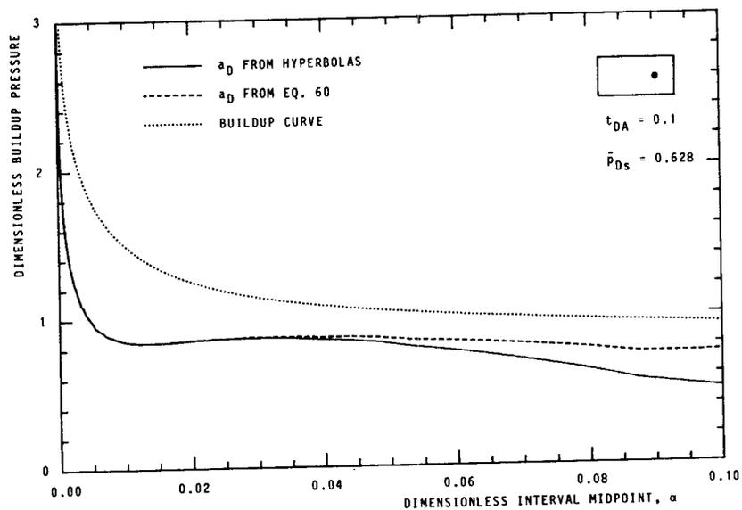
Fig. 17—Asymptotes from hyperbolas and Eq. 60 compared with buildup curve following nonstabilized flow for a closed 2:1 rectangle.
