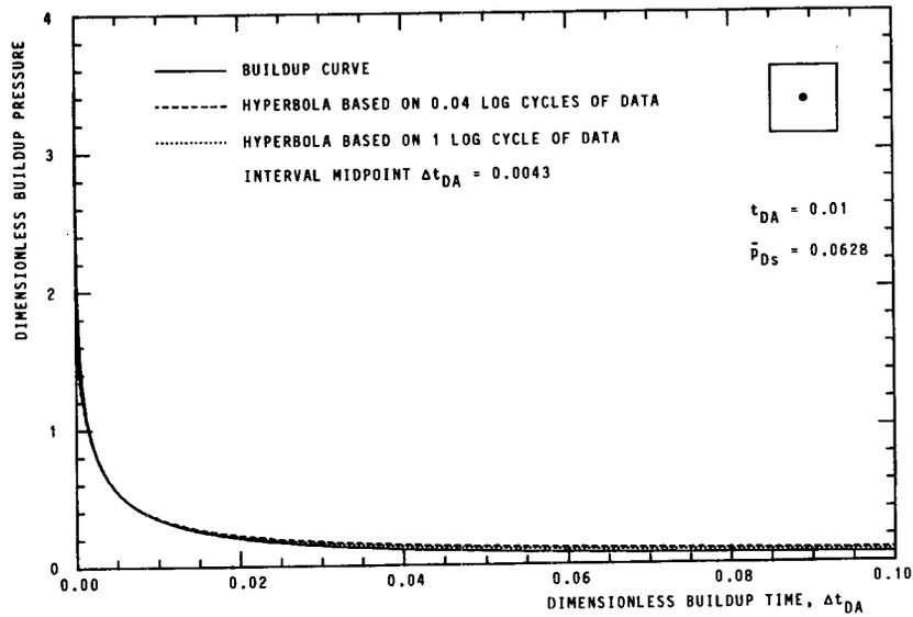
Fig. 1—Effect of interval length when hyperbolas are matched to buildup curves.
