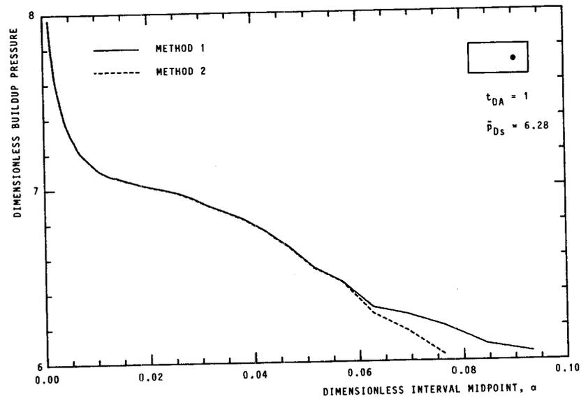
Fig. 20—A comparison of Methods 1 and 2 to determine asymptotes of hyperbolas matched to buildup data of a closed 2:1 rectangle.
