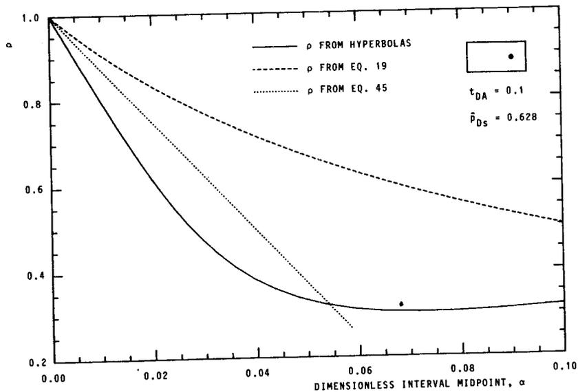
Fig. 19—Slope parameter  $\rho$  from hyperbolas and Eqs. 19 and 45 following nonstabilized flow for a closed 2:1 rectangle.
