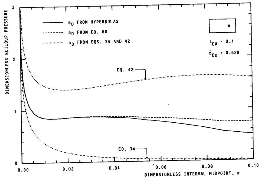
Fig. 18—Asymptotes from hyperbolas and Eqs. 34, 42, and 60 following nonstabilized flow for a closed 2:1 rectangle.
