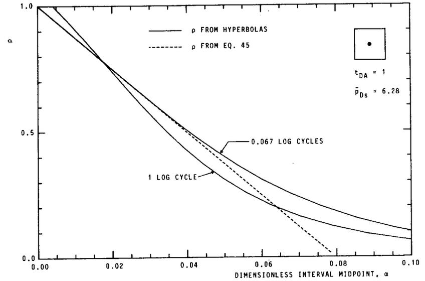
Fig. 6—Slope parameter  $\rho$  from hyperbolas and Eq. 45 for a closed square produced to pseudosteady state prior to shut-in.
