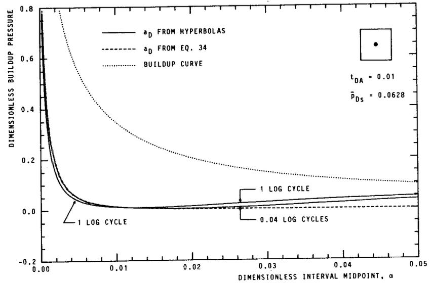
Fig. 2—Asymptotes from hyperbolas and Eq. 34 compared with buildup curve of an infinite-acting reservoir.
