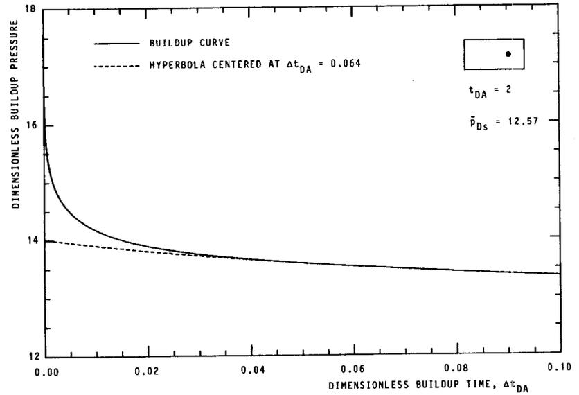
Fig. 8—Hyperbola with asymptote given by average pressure matched to buildup curve following pseudosteady-state flow for a closed 2:1 rectangle.
