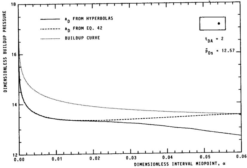
Fig. 7—Asymptotes from hyperbolas and Eq. 42 compared with buildup curve following pseudosteady-state flow for a closed 2:1 rectangle.
