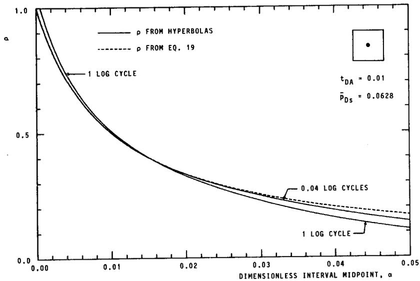
Fig. 3—Slope parameter  $\rho$  from hyperbolas and Eq. 19 for an infinite-acting reservoir.
