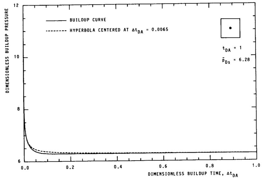
Fig. 4—Hyperbola matched to buildup curve of a closed square produced to pseudosteady state prior to shut-in.
