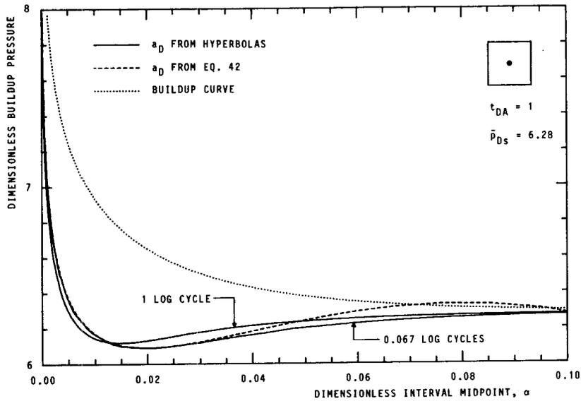
Fig. 5—Asymptotes from hyperbolas and Eq. 42 compared with buildup curve following pseudosteady-state flow for a closed square.
