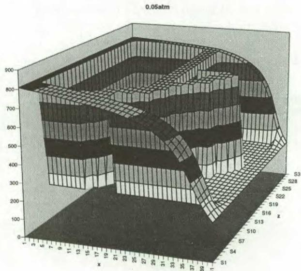
Figure 2. Water saturation distribution at pressure drop 0.05 atm
