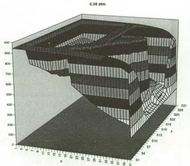
Figure 3. Water saturation distribution at pressure drop 0.38 atm.
