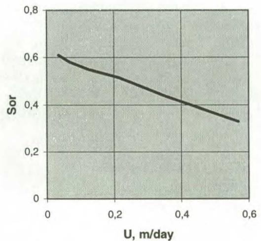
Figure 4. Capillary trapped oil as a function of total rate
