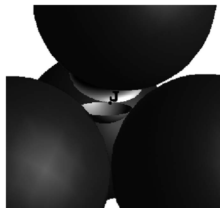
Fig. 18. At a smaller value of curvature than in Fig. 17, the ring and meniscus first come into contact at point J. This results in the instability of the interface and leads to the imbibition event: all NW phase withdraws and W phase completely fills the pore.
