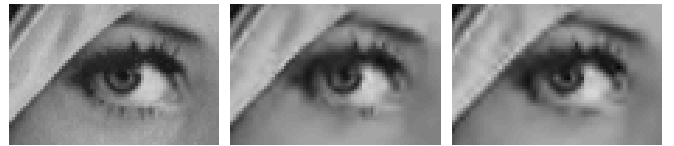
Fig. 2. A detail from the test image lena . Original to the left, RLS-DLA (PSNR = 35.26) in the middle and SPITH (PSNR = 34.78) to the right. 0.25 bits per pixel. Some differences can be seen in the lower eyelash.
