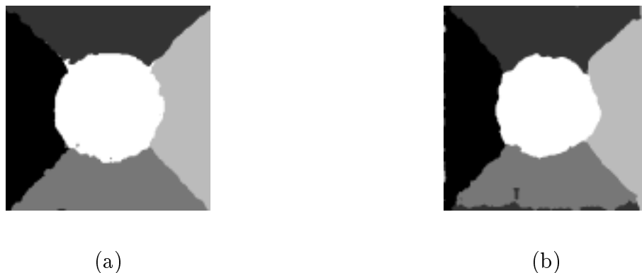
Figure 3.1: Segmentation results with the texture mosaic of Figure 1.1(a) and different Gabor filter approaches, (a) with the decomposition of Jain and Farrokhnia [50] and (b) with the sub-band decomposition of Figure 2.6(d).
