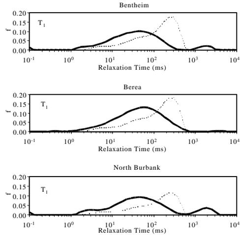
Fig. 15 T<sub>1</sub> relaxation time distributions of the sandstones after D<sub>2</sub>O brine diffusion (solid curve) compared to bulk SMY crude oil (dotted curve), scaled to oil saturation.
