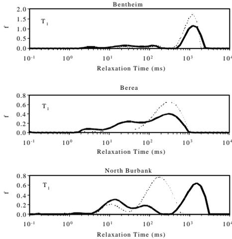
Fig. 14 T<sub>1</sub> relaxation time distributions of the sandstones after forced imbibition (solid curve) compared to 100% brine saturation (dotted curve).
