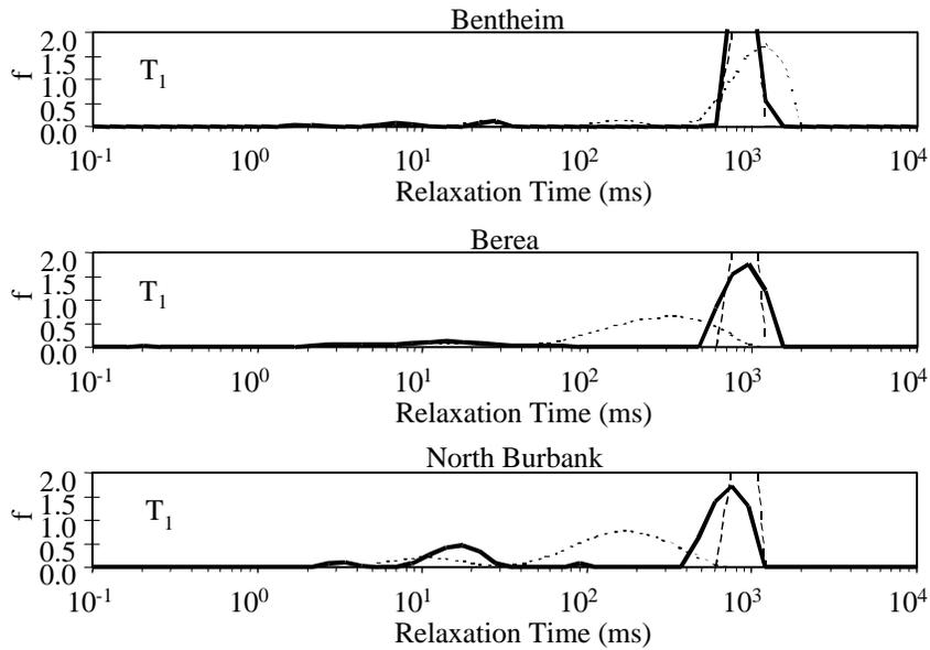
Fig. 4  $T_1$  relaxation time distributions of the sandstones at 100% brine saturation (dotted curve) and Soltrol saturated to  $S_{wir}$  (solid curve). The  $T_1$  relaxation time distribution of bulk Soltrol is shown as the dashed curve.
