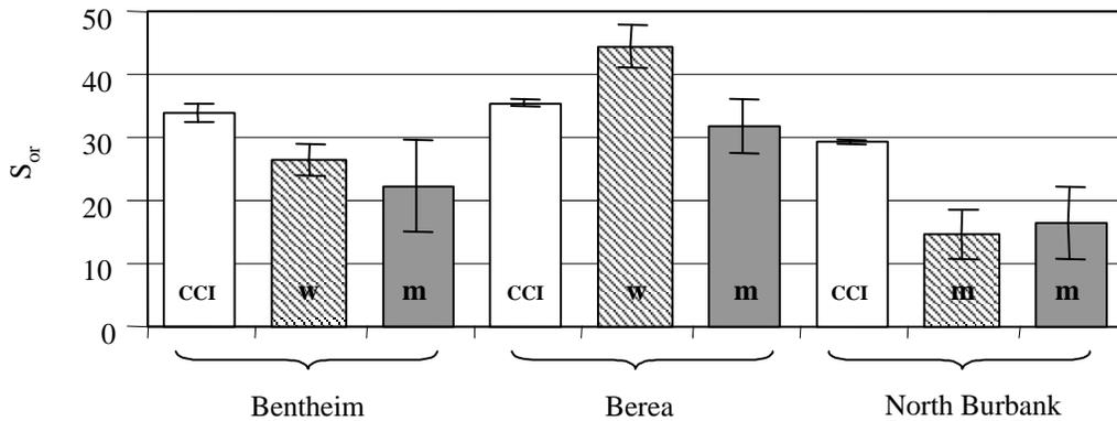
Fig. 17 Residual oil saturation from CCI (white bars), refined oil systems (hashed bars) and crude oil systems (shaded bars).
