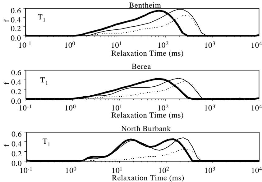
Fig. 10  $T_1$  relaxation time distributions of the sandstones with SMY crude oil saturated to  $S_{wir}$  before aging (solid curve) and after aging (bold solid curve). The  $T_1$  relaxation time distribution of bulk SMY crude oil, scaled to oil saturation, is shown as the dotted curve.
