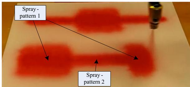
**Fig. 3.** Painting on paper allows for the visual inspection of the timing of different actuator outputs. However, the inspection must typically be performed by a paint process engineer in cooperation with a software engineer.
