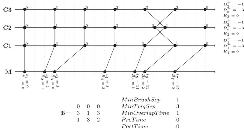
**Fig. 9.** An optimal solution for Exp1a. The cost function used by the solver is *minimize*( $t_7$ ), where the optimal solution is  $t_7 = 15$ . The number next to each black dot (●) represents the value of the actuator output to apply at that time instance. The configuration of each actuator output is to the right of each actuator output's time axis ( $D^+$ ,  $D^-$ , and  $K$ ).
