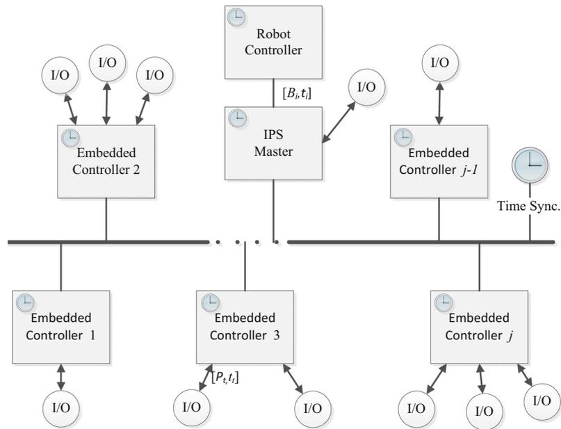
**Fig. 2.** Logical overview of the IPS. The IPS is interconnected by an industrial-grade network. All the embedded boards are synchronized by use of IEEE 1588 [16]. Each embedded controller is typically located inside the robot's control cabinet, at different locations on the robot arm, or in an external process control cabinet.
