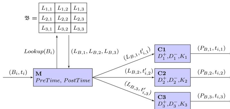
Fig. 8. Logical overview of experiment Exp1a. The experiment includes the use of three actuator outputs (channels), a test sequence of length 7 ( $SeqLen$ ), and a lookup table size of size 3 ( $|\mathfrak{B}|$ ).
