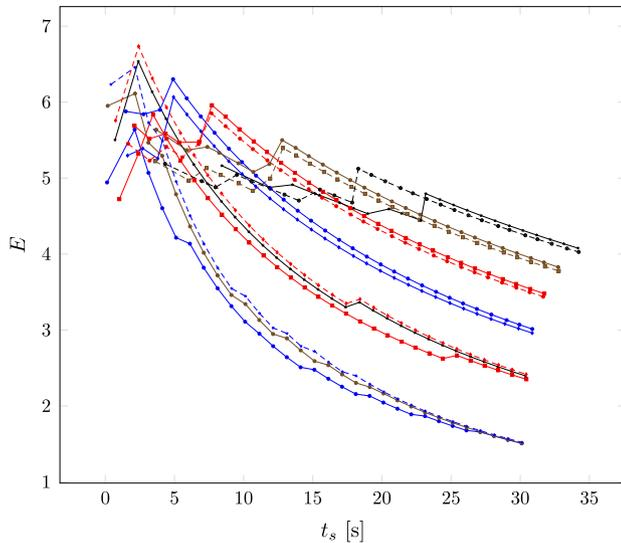
**Fig. 12.** Efficiency factor  $E$  for the executions in Fig. 11. When the model is run in a continuous integration environment, there is little to gain from running the model more than around 10 s.
