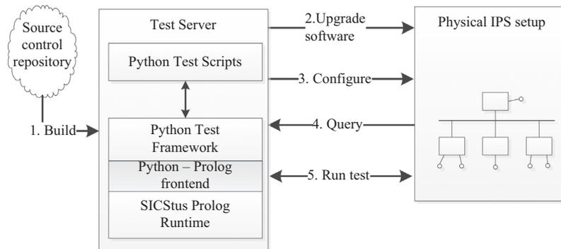
Fig. 6. Integration between the test server and IPS. The test server typically receives a new build from a build server, upgrades all embedded boards, performs tests, and publishes the results for the developer. The numbers correspond to the explanation given in Section 7.1.
