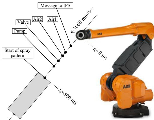
Fig. 1. To achieve the correct spray pattern at the starting edge of the object to be painted, different physical processes need to be activated with individual timing before the robot reaches the object.
