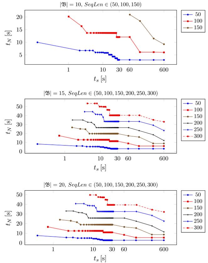
**Fig. 11.** How well the model minimizes the duration of the test sequence,  $t_N$ , if more time is added to the solving process,  $t_s$ .
