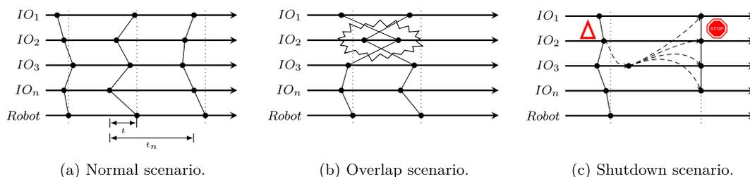
**Fig. 5.** A collection of error scenarios that the model can generate. Horizontal lines represent time and a black dot represents the activation of an output. A specific *spray pattern* is a collection of output activations, visualized by a line connecting the black dots.
