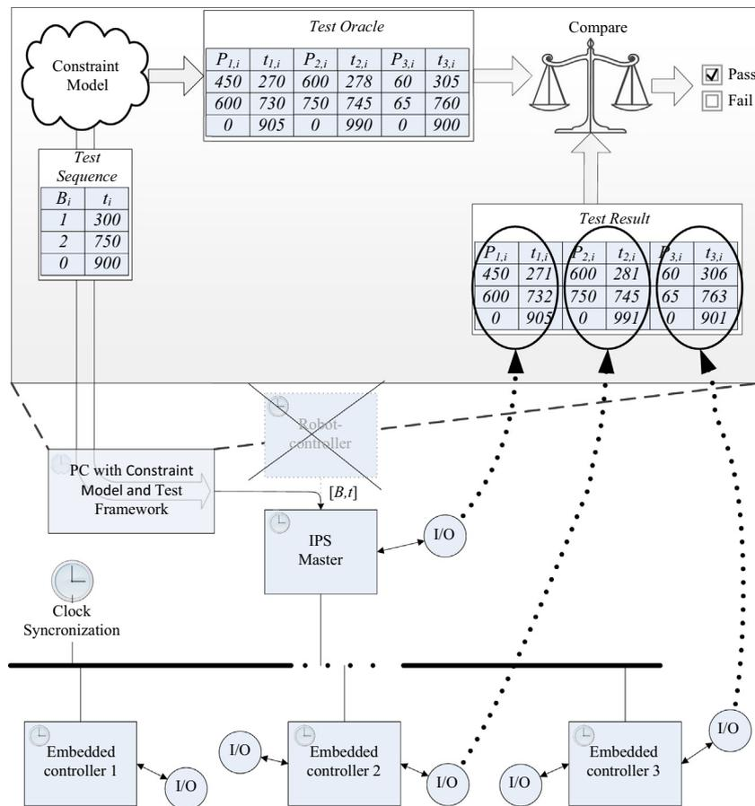
**Fig. 7.** How a complete test is executed. The constraint model generates the test sequence, the configuration of the IPS, and the oracle. The configuration is applied to the IPS and the test sequence is executed. The oracle is then compared with actual measurements before a pass/fail is determined. Currently 11 different variations of this setup are being executed in parallel at ABB Robotics.
