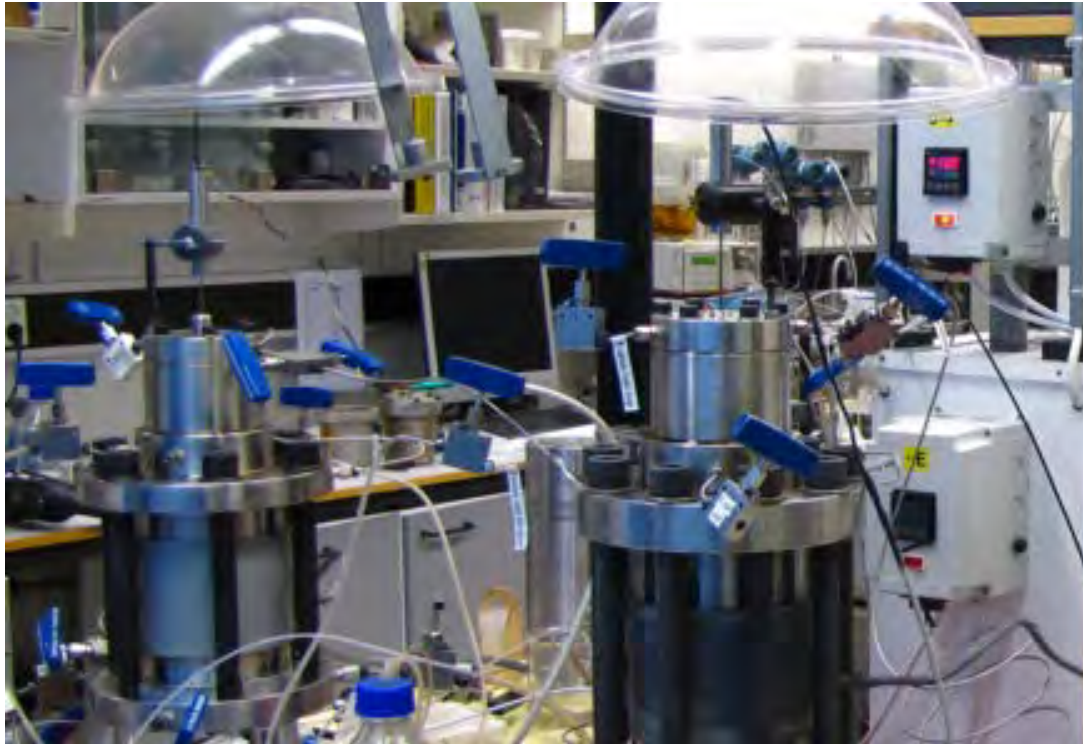
Figure: Triaxial cells at UiS laboratory where the rock is exposed to mechanical compression tests under reservoir conditions ( www.uis.no ).
