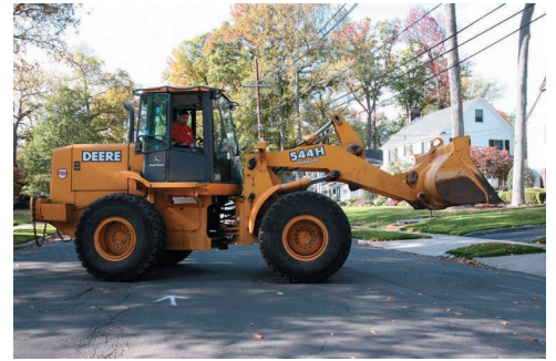
Photo 4.1 A free-body diagram of the tractor shown would include all of the external forces acting on the tractor: the weight of the tractor, the weight of the load in the bucket, and the forces exerted by the ground on the tires.
