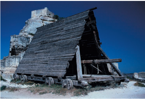
Photo 15.1 This replica of a battering ram at Château des Baux , France undergoes curvilinear translation.
