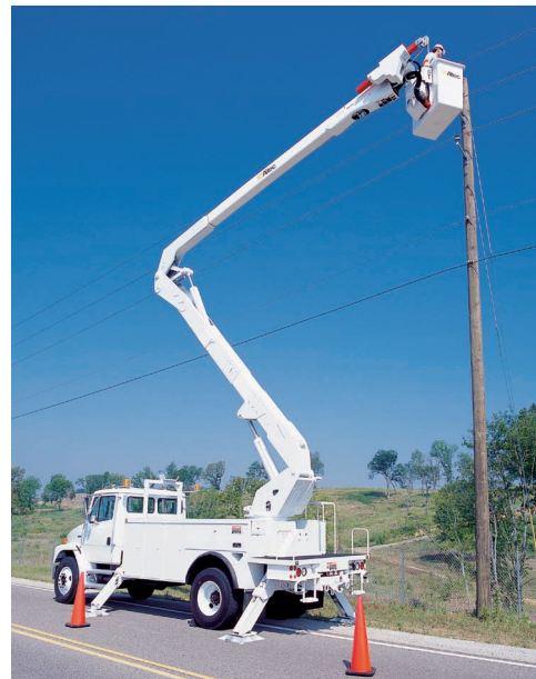
Photo 10.1 The forces exerted by the hydraulic cylinders to position the bucket lift shown can be effectively determined using the method of virtual work since a simple relation exists among the displacements of the points of application of the forces acting on the members of the lift.
