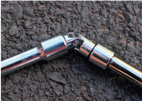
Photo 4.6 Universal joints, easily seen on the drive shafts of rear-wheel-drive cars and trucks, allow rotational motion to be transferred between two noncollinear shafts.
