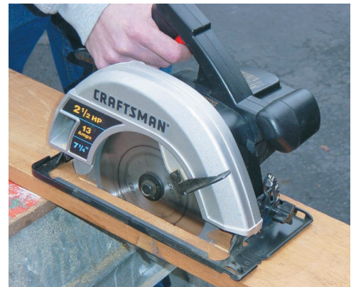
Photo 7.1 The design of the shaft of a circular saw must account for the internal forces resulting from the forces applied to the teeth of the blade. At a given point in the shaft, these internal forces are equivalent to a force-couple system consisting of axial and shearing forces and a couple representing the bending and torsional moments.
