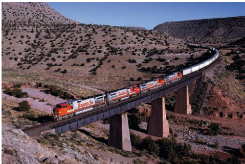
Photo 11.5 The passengers in a train traveling around a curve will experience a normal acceleration toward the center of curvature of the path.
