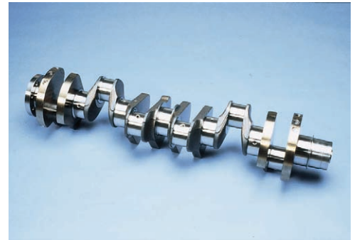
Photo 18.4 The forces exerted by a rotating automobile crankshaft on its bearings are the static and dynamic reactions. The crankshaft can be designed to be dynamically as well as statically balanced.
