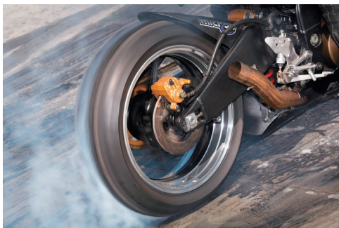
Photo 17.1 The work done by friction reduces the kinetic energy of the wheel.
