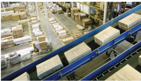
Photo 8.1 The coefficient of static friction between a package and the inclined conveyor belt must be sufficiently large to enable the package to be transported without slipping.
