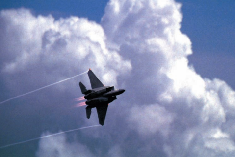
Photo 12.2 The pilot of a fighter aircraft will experience very large normal forces when taking a sharp turn.
