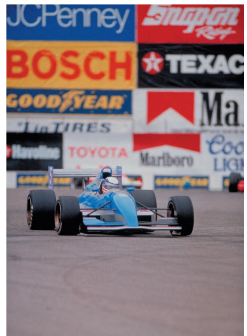
Photo 12.1 When the racecar accelerates forward the rear tires have a friction force acting on them in the direction the car is moving.
