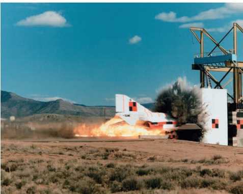
Photo 13.2 This impact test between an F-4 Phantom and a rigid reinforced target was to determine the impact force as a function of time.
