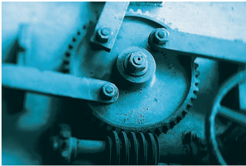
Photo 15.6 The central gear rotates about a fixed axis and is pin-connected to three bars which are in general plane motion.
