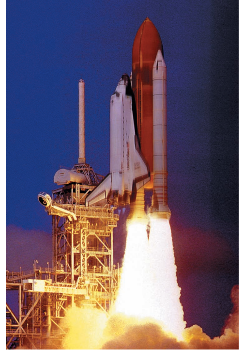
Photo 14.3 As the shuttle's booster rockets are fired, the gas particles they eject provide the thrust required for liftoff.
