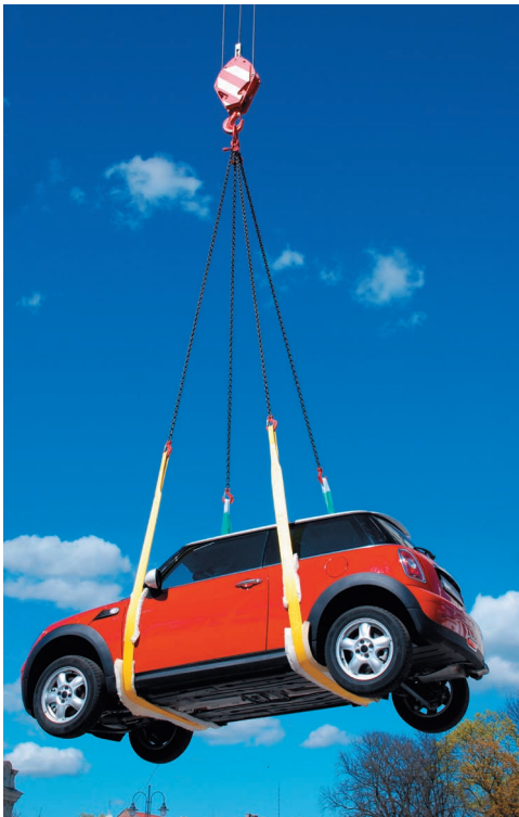
Photo 2.2 While the tension in the four cables supporting the car cannot be found using the three equations of (2.34), a relation between the tensions can be obtained by considering the equilibrium of the hook.
