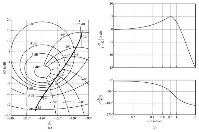
Figure 7–85 (a) Plot of  $G(j\omega)$  superimposed on Nichols chart; (b) closed-loop frequency-response curves.
