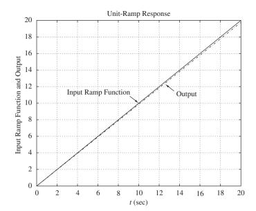
Figure 8–56 Unit-ramp response of C(s)/R(s) =  $(6.104s^2 + 40.6104s +$   $4)/(s^3 + 6.104s^2 +$ 41.6104s + 4).
