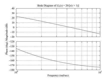
**Figure 7–146** Bode diagram of  $G_1(s)$ .
