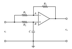
**Figure 3–26** Operational-amplifier circuit.
