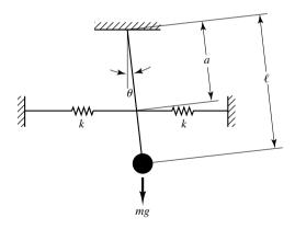
Figure 3–33 Spring-loaded pendulum system.
