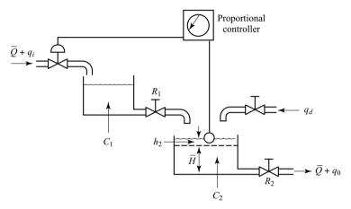
**Figure 4–43** Liquid-level control system.
