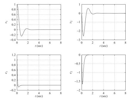
Figure 10–52 Response curves to initial condition.
