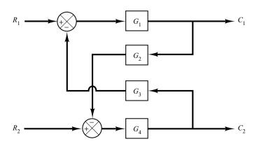
**Figure 2–24** System with two inputs and two outputs.
