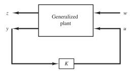
**Figure 10–48** A generalized plant diagram.
