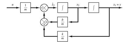
Figure 2–16 Block diagram of the mechanical system shown in Figure 2–15.
