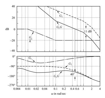
Figure 7–104 Bode diagrams for  $G_1$  (gain-adjusted but uncompensated open-loop transfer function),  $G_c$  (compensator), and  $G_cG$  (compensated open-loop transfer function).
