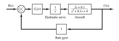
**Figure 6–94**Compensated attitude-rate control system.
