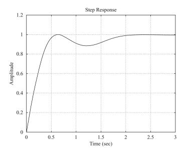
Figure 5–56 Unit-step response curve.
