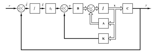
**Figure 10–6** Type 1 servo system.
