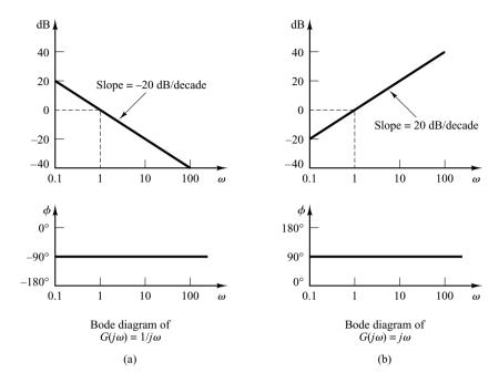
Figure 7-5 (a) Bode diagram of  $G(j\omega) = 1/j\omega$ ; (b) Bode diagram of  $G(j\omega) = j\omega$ .
