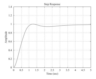
Figure 8–21 Unit-step response of the system with K = 2.8 and a = 0.7. (The maximum overshoot is 0.24%.)
