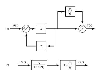
Figure 2–18 Simplified block diagrams for the system shown in Figure 2–17.
