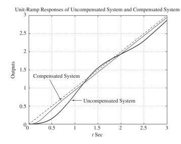
Figure 7–150 Unit-ramp responses of the uncompensated and compensated systems.
