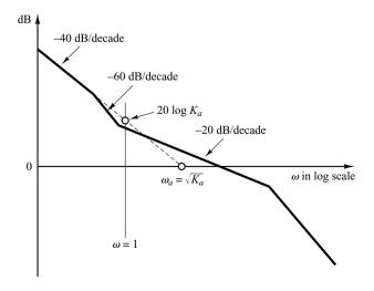
**Figure 7–19** Log-magnitude curve of a type 2 system.
