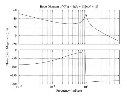
**Figure 8–15** Bode diagram of  $G(s) = 4(5s + 1)/[s(s^2 + 1)].$
