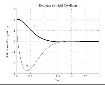
**Figure 5–32** Response of system in Example 5–9 to initial condition.
