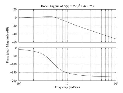
Figure 7–20 Bode diagram of  $G(s) = \frac{25}{s^2 + 4s + 25}.$
