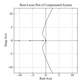
**Figure 6–78**Root-locus plot of the compensated system.
