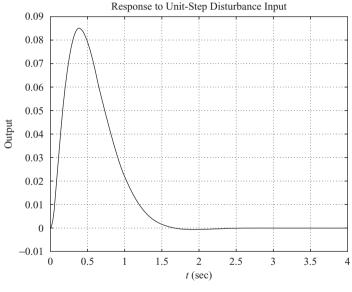
Figure 8–36 (a) Response to unit-step reference input (a = 3.2, b = 2, c = 12); (b) response to unit-step disturbance input (a = 3.2, b = 2, c = 12).
