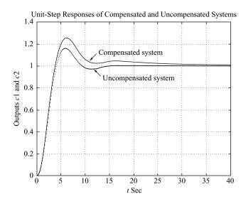
Figure 6–52 Unit-step responses of compensated and uncompensated systems. [The compensator is given by Equation (6–20).]
