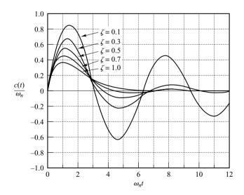
Figure 5–14 Unit-impulse response curves of the system shown in Figure 5–6.
