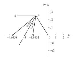
Figure 6–42 Determination of the pole and zero of the lead compensator.
