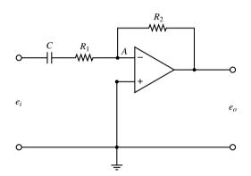
Figure 3–39 Operational-amplifier circuit.
