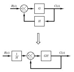
Figure 7–62 Modification of a system with feedback elements to a unityfeedback system.
