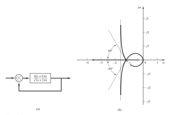
**Figure 6–66**(a) Control system; (b) root-locus plot.
