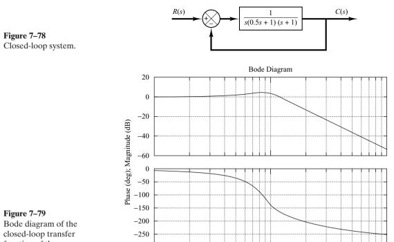
Bode diagram of the closed-loop transfer function of the system shown in Figure 7–78.
