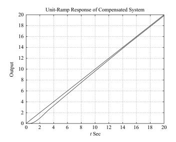
Figure 7–114 Unit-ramp response of the compensated system (Example 7–28).
