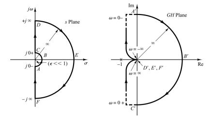
Figure 7-51 s-Plane contour and the G(s)H(s) locus in the GHplane, where G(s)H(s) = K/[s(Ts+1)].
