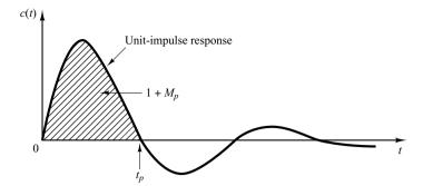
Figure 5–15 Unit-impulse response curve of the system shown in Figure 5–6.
