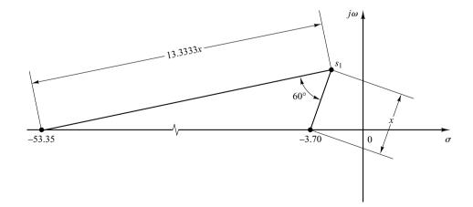
Figure 6–87 Graphical determination of the zero and pole of the lead portion of the compensator.
