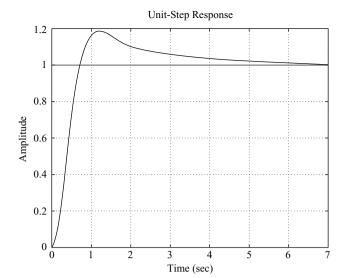
**Figure 8–9** Unit-step response of the system shown in Figure 8–6 with PID controller having parameters  $K_p = 18$ ,  $T_i = 3.077$ , and  $T_d = 0.7692$ .
