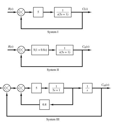
**Figure 5–77**Positional servo system (System I), positional servo system with PD control action (System II), and positional servo system with velocity feedback (System III).
