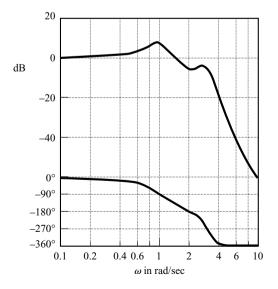
Figure 7–143 Bode diagram of G(s)/[1 + G(s)], where G(s) is given by Equation (7–32).
