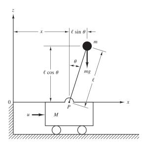
**Figure 3–6** Inverted-pendulum system.
