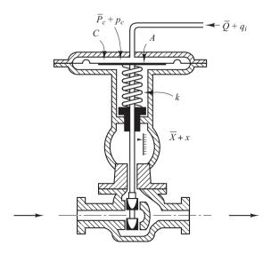
Figure 4–11 Schematic diagram of a pneumatic actuating valve.
