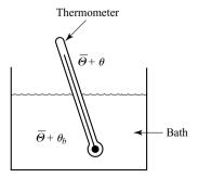
Figure 4–40 Thin, glass-wall, mercury thermometer system.
