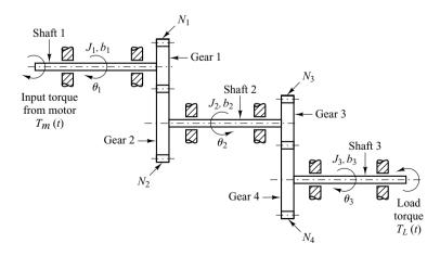
**Figure 5–51** Gear-train system.
