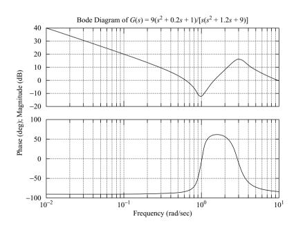
Figure 7-22 Bode diagram of  $G(s) = \frac{9(s^2 + 0.2s + 1)}{s(s^2 + 1.2s + 9)}.$
