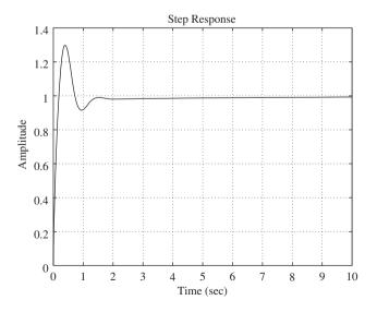
Figure 8-55 Unit-step response of  $C(s)/R(s) = (6.104s^2 + 40.6104s + 4)/(s^3 + 6.104s^2 + 41.6104s + 4)$ .
