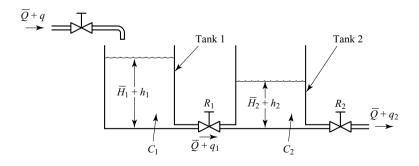
Figure 4–2 Liquid-level system with interaction.
