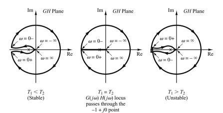
**Figure 7–55**Polar plots of the system considered in Example 7–16.
