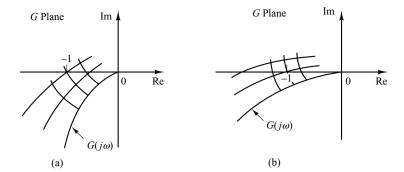
**Figure 7–65** Conformal mappings of *s*-plane grids for the systems shown in Figure 7–64 into the G(s) plane.
