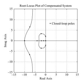
**Figure 6–96**Root-locus plot of the compensated system.
