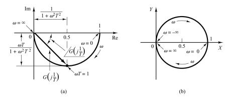
Figure 7-26 (a) Polar plot of  $1/(1 + j\omega T)$ ; (b) plot of  $G(j\omega)$  in X-Yplane.
