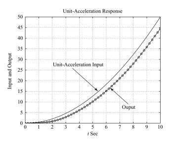
**Figure 5–63** Response to unitacceleration input.
