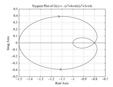
**Figure 7–130** Nyquist plot for positive-feedback system.
