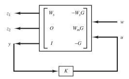
**Figure 10–47** Generalized plant of the system discussed in Example 10–15.
