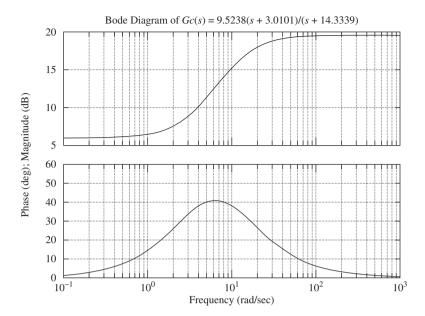
**Figure 7–147** Bode diagram of  $G_c(s)$ .
