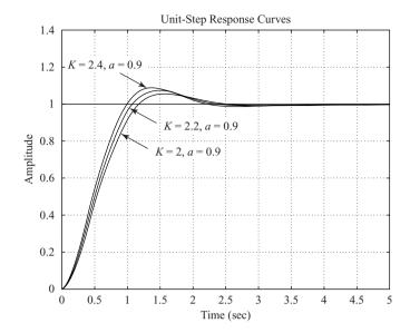
Figure 8–22 Unit-step response curves of system with K = 2, a = 0.9; K = 2.2, a = 0.9; and K = 2.4, a = 0.9.
