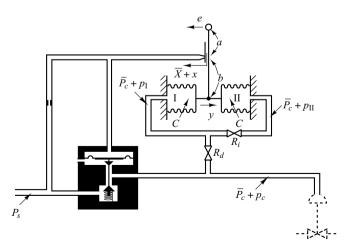
**Figure 4–30** Schematic diagram of a pneumatic controller.
