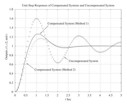
Figure 6–45 Unit-step response curves of designed systems and original uncompensated system.
