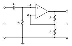
Figure 3–40 Operational-amplifier circuit.
