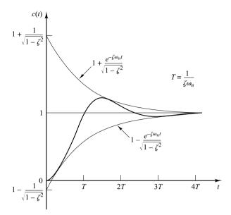
Figure 5–10 Pair of envelope curves for the unitstep response curve of the system shown in Figure 5–6.
