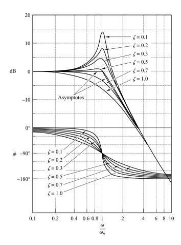
Figure 7–9 Log-magnitude curves, together with the asymptotes, and phase-angle curves of the quadratic transfer function given by Equation (7–7).
