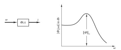
Figure 10–41 Bode diagram and the  $H_{\infty}$  norm  $\|\Phi\|_{\infty}$ .
