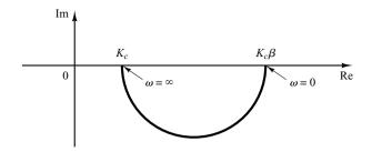
Figure 7–101 Polar plot of a lag compensator  $K_c\beta(j\omega T + 1)/(j\omega\beta T + 1)$ .
