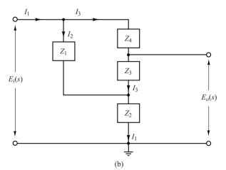
**Figure 3–25**(a) Bridged *T*network in terms of complex impedances;
