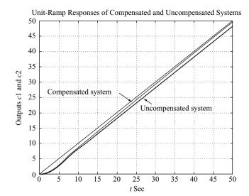
Figure 6–51 Unit-ramp responses of compensated and uncompensated systems. [The compensator is given by Equation (6–20).]
