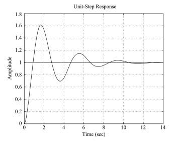
Figure 8–8 Unit-step response curve of PIDcontrolled system designed by use of the Ziegler–Nichols tuning rule (second method).
