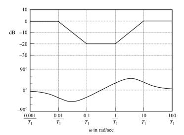
**Figure 7–110** Bode diagram of a lag–lead compensator given by Equation (7–27) with  $K_c = 1$ ,  $\gamma = \beta = 10$ , and  $T_2 = 10T_1$ .
