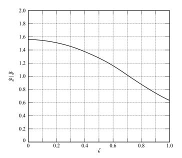
**Figure 7–134** Curve of  $\omega_b/\omega_n$  versus  $\zeta$ , where  $\omega_b$  is the bandwidth.
