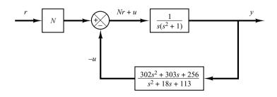
Figure 10–31 Control system with observer controller in the feedback path.
