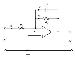
**Figure 3–16** First-order lag circuit using operational amplifier.
