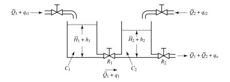
Figure 4–28 Liquid-level system.
