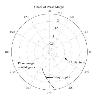
Figure 7–140 Nyquist plot of  $G(j\omega)$  showing that the phase margin is  $60^{\circ}$ .
