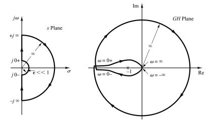
Figure 7–52 s-Plane contour and the G(s)H(s) locus in the GH plane, where  $G(s)H(s) = K/[s^2(Ts+1)]$ .
