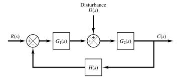
Figure 2–11 Closed-loop system subjected to a disturbance.
