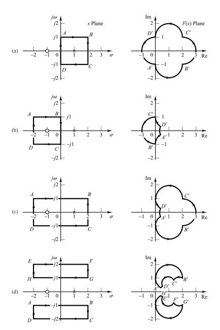
Figure 7–46 Closed contours in the s plane and their corresponding closed curves in the F(s) plane, where F(s) = (s + 1)/(s - 1).
