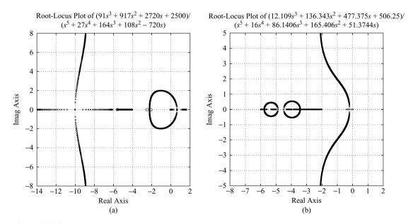
Figure 10–24 (a) Root-locus plot of the system with observer poles at s = -10 and s = -10; (b) root-locus plot of the system with observer poles at s = -4.5 and s = -4.5.
