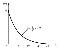
Figure 5–4 Unit-impulse response of the system shown in Figure 5–1(a).
