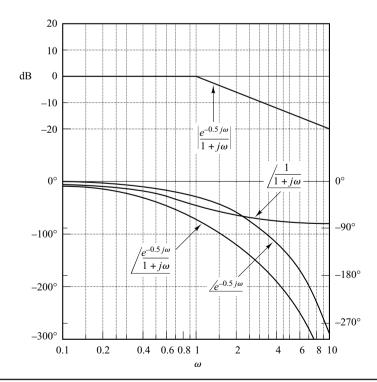
**Figure 7–15** Bode diagram for the system  $e^{-j\omega L}/(1 + j\omega T)$  with L = 0.5 and T = 1.
