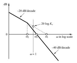
**Figure 7–18** Log-magnitude curve of a type 1 system.
