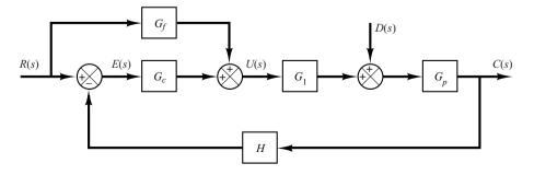
Figure 2–23 Control system with reference input and disturbance input.
