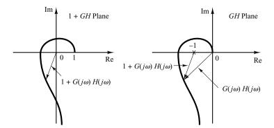
Figure 7–48 Plots of  $1 + G(j\omega)H(j\omega)$  in the 1 + GH plane and GH plane.
