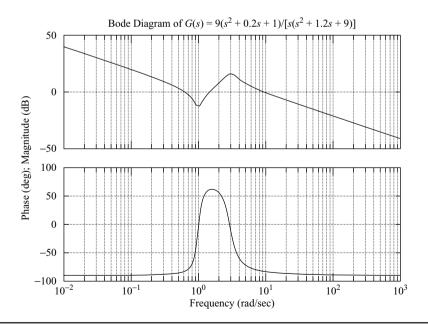
Figure 7-23 Bode diagram of  $G(s) = \frac{9(s^2 + 0.2s + 1)}{s(s^2 + 1.2s + 9)}$
