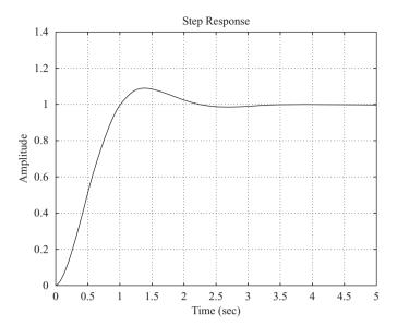
Figure 8–20 Unit-step response of the system with K = 2.4 and a = 0.9. (The maximum overshoot is 9.23%.)
