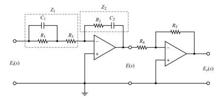
**Figure 8–45** Modified PID controller.
