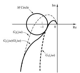
**Figure 7–90**Reshaping of the open-loop frequency-response curve.
