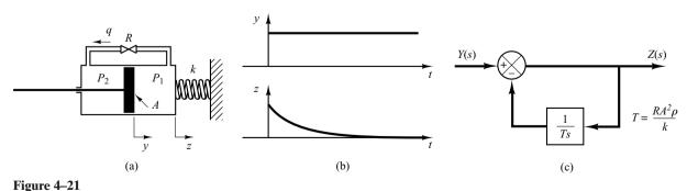
(a) Dashpot; (b) step change in y and the corresponding change in z plotted versus t; (c) block diagram of the dashpot.
