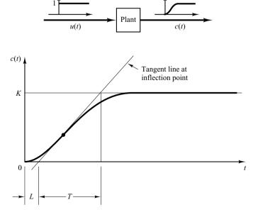
**Figure 8–3** S-shaped response curve.
