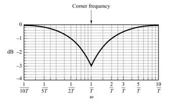
**Figure 7–7** Log-magnitude error in the asymptotic expression of the frequency-response curve of  $1/(1 + j\omega T)$ .
