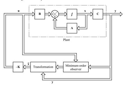
Figure 10–16 Observed-state feedback control system with a minimum-order observer.
