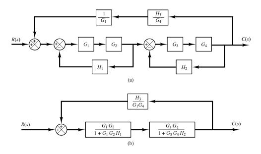
Figure 2–22 Successive reductions of the block diagram shown in Figure 2–21.
