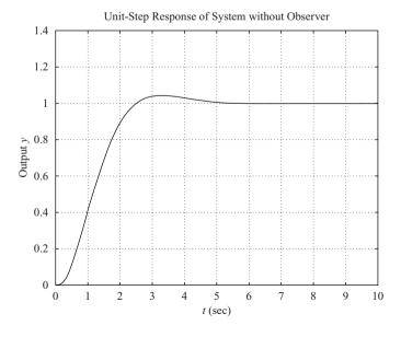
Figure 10–33 The unit-step response of the control system designed by the pole placement approach without observer. (The closed-loop poles are at  $s = -1 \pm j$ , s = -8.)
