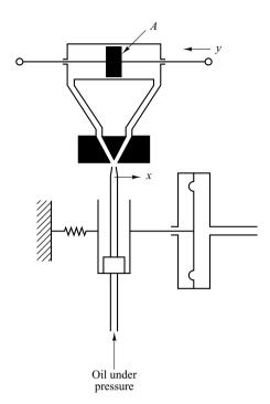
**Figure 4–34** Hydraulic jet-pipe controller.
