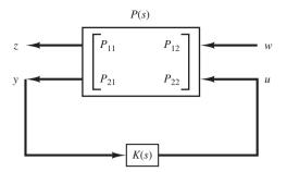
**Figure 10–46** A generalized plant diagram.
