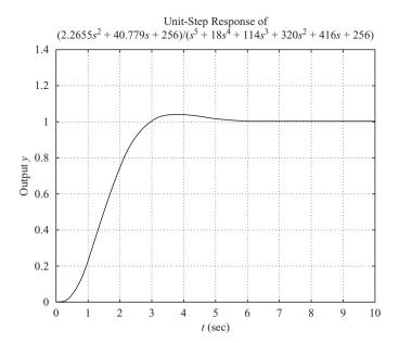
Figure 10–32 The unit-step response of the system shown in Figure 10–31. (The closed-loop poles for pole placement are at  $s = -1 \pm j$ , s = -8. The observer poles are at s = -4, s = -4.)
