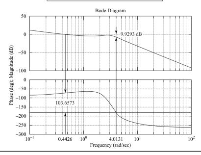
**Figure 7–72** Bode diagram of G(s) shown in Figure 7–71.
