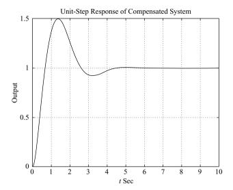
Figure 6–79 Unit-step response of the compensated system.
