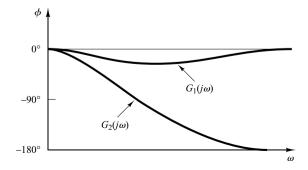
Figure 7–13 Phase-angle characteristics of the systems  $G_1(s)$  and  $G_2(s)$  shown in Figure 7–12.
