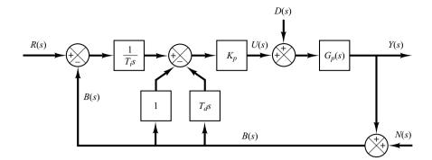
**Figure 8–27** I-PD-controlled system.
