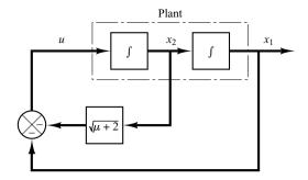
Figure 10–37 Optimal control of the plant shown in Figure 10–36.
