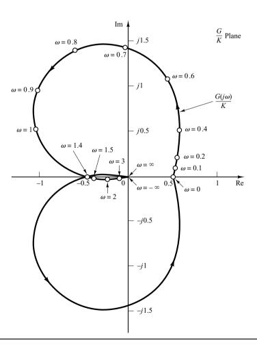
Figure 7–61 Polar plot of  $G(j\omega)/K$ .
