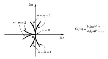
**Figure 7–34**Polar plots in the high-frequency range.
