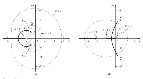
Figure 6-29 Plots of root loci and constant-gain loci. (a) System with  $G(s) = K(s+2)/(s^2+2s+3)$ , H(s) = 1; (b) system with G(s) = K/[s(s+1)(s+2)], H(s) = 1.
