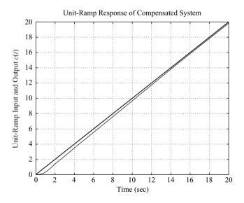
Figure 7–155 Unit-ramp response of the compensated system.
