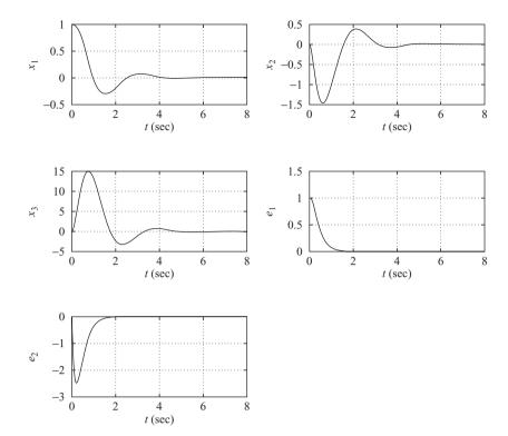
Figure 10–21 Response to the given initial condition;  $x_1(0) = 1$ ,  $x_2(0) = 0$ ,  $x_3(0) = 0$ ,  $e_1(0) = 1$ ,  $e_2(0) = 0$ .
