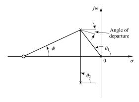
Figure 6–12 Construction of the root locus. [Angle of departure =  $180^{\circ} - (\theta_1 + \theta_2) + \phi$ .]
