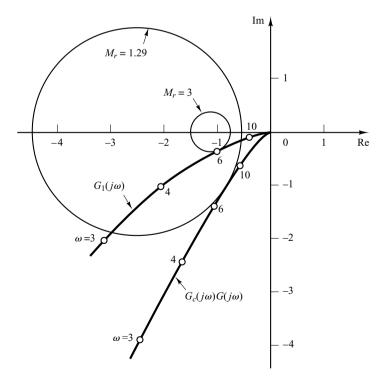
Figure 7–98 Polar plots of the gain-adjusted but uncompensated open-loop transfer function  $G_1$  and compensated open-loop transfer function  $G_cG$ .
