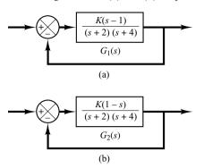
Figure 6–102 (a) and (b) Nonminimum-phase systems.
