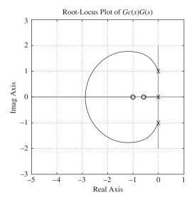
**Figure 8–50** Root-locus plot of the compensated system.
