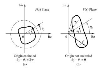
Figure 7–122 Determination of encirclement of the origin of F(s) plane.
