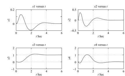
Figure 10–10 Curves  $x_1$  versus t,  $x_2$  versus t,  $x_3$ (= output y) versus t,  $x_4$  versus t, and  $x_5$  (=  $\xi$ ) versus t.
