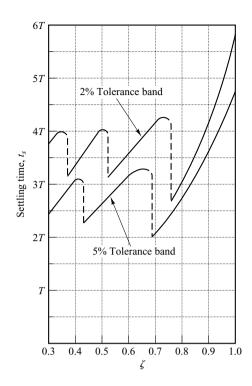
Figure 5–11 Settling time  $t_s$  versus  $\zeta$  curves.
