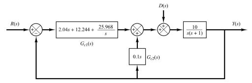
**Figure 8–37** Block diagram of the designed system.
