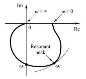
Figure 7–29 Polar plot showing the resonant peak and resonant frequency  $\omega_r$ .
