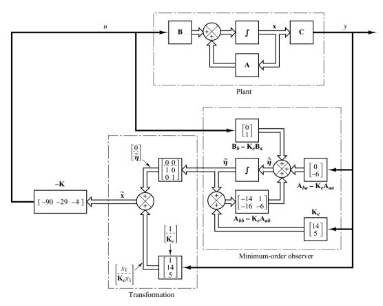
**Figure 10–18**System with observed state feedback, where the observer is the minimum-order observer designed in Example 10–8.
