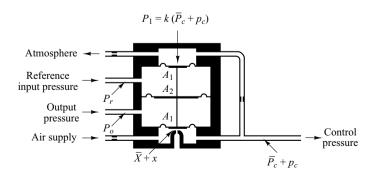
Figure 4–10 Schematic diagram of a force-balance type pneumatic proportional controller.
