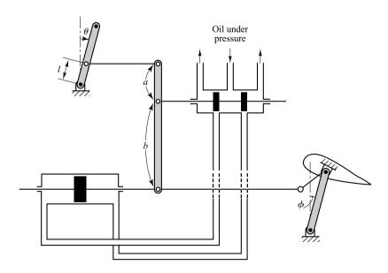
**Figure 4–51** Aircraft elevator control system.
