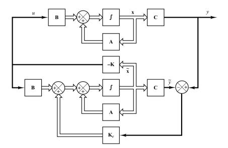
Figure 10–12 Observed-state feedback control system.
