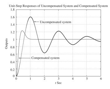
Figure 7–149 Unit-step responses of the uncompensated and compensated systems.
