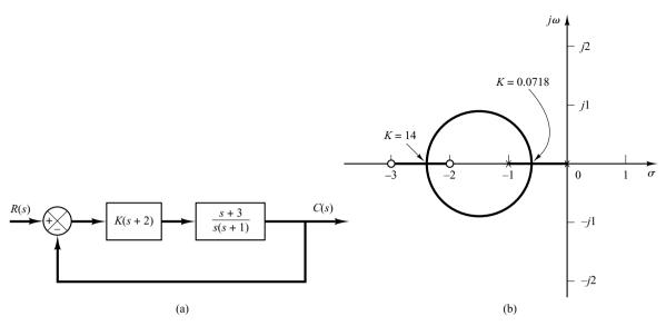
**Figure 6–64**(a) Control system; (b) root-locus plot.
