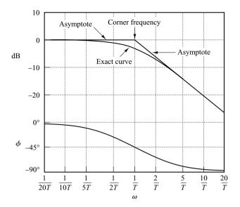
Figure 7–6 Log-magnitude curve, together with the asymptotes, and phase-angle curve of  $1/(1 + j\omega T)$ .
