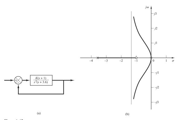
**Figure 6–65**(a) Control system; (b) root-locus plot.
