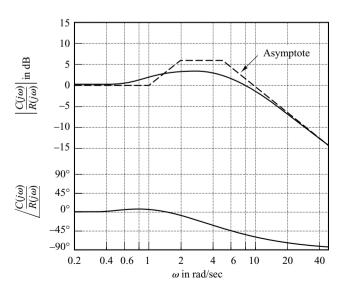
Figure 7–118 Bode diagram for  $10(1 + j\omega)/[(2 + j\omega)(5 + j\omega)]$ .
