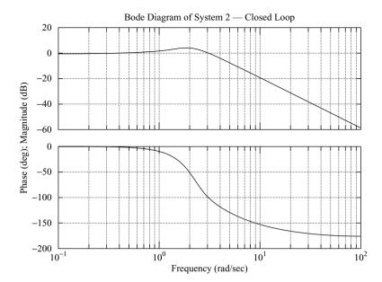
Figure 10–23 Bode diagram for the closed-loop transfer function of System 2.
