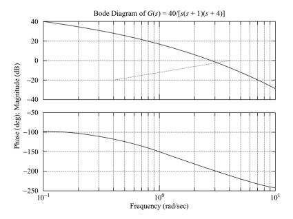
Figure 7–151 Bode diagram of G(s) = 40/[s(s+1)(s+4)].
