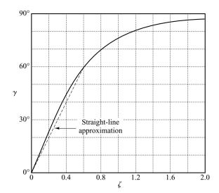
Figure 7–74 Curve  $\gamma$  (phase margin) versus  $\zeta$  for the system shown in Figure 7–73.
