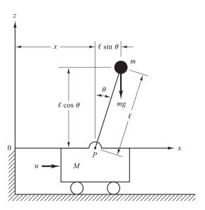
Figure 10–8 Inverted-pendulum control system.
