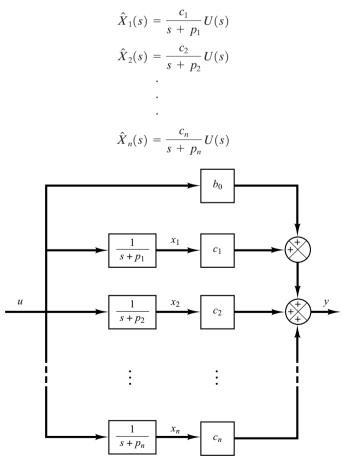
Figure 9–3 Block diagram representation of the system defined by Equations (9–84) and (9–85) (diagonal canonical form).
