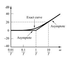
Figure 7–8 Log-magnitude curve, together with the asymptotes, and phase-angle curve for  $1 + j\omega T$ .
