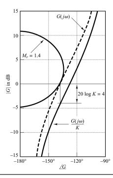
**Figure 7–86** Determination of the gain *K* using the Nichols chart.
