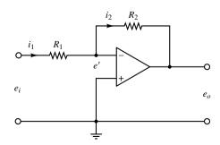
**Figure 3–14** Inverting amplifier.
