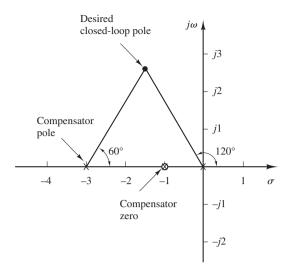
**Figure 6–44** Compensator pole and zero.
