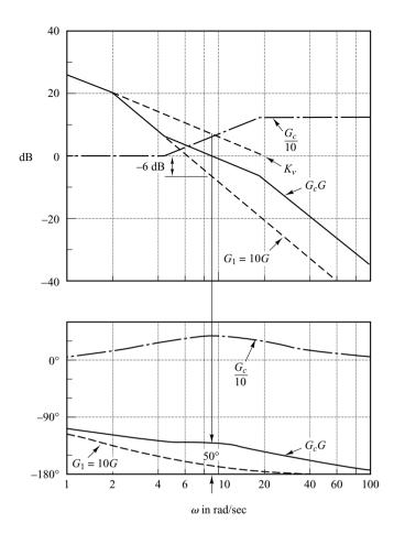
**Figure 7–96**Bode diagram for the compensated system.
