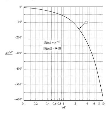
Figure 7–14 Phase-angle characteristic of transport lag.
