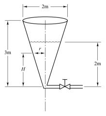
Figure 4-42 Conical water-tank system.
