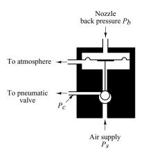
**Figure 4–7** Reverse-acting relay.
