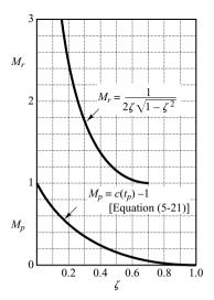
**Figure 7–75** Curves  $M_r$  versus  $\zeta$  and  $M_p$  versus  $\zeta$  for the system shown in Figure 7–73.
