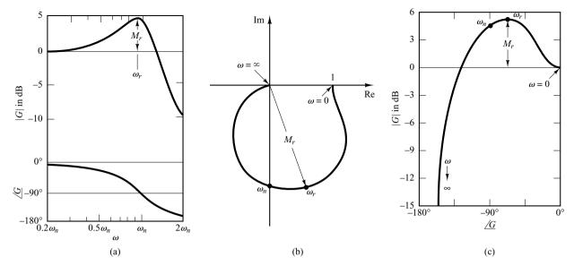
Figure 7–43 Three representations of the frequency response of  $\frac{1}{1+2\zeta\Big(j\frac{\omega}{\omega_n}\Big)+\Big(j\frac{\omega}{\omega_n}\Big)^2}, \text{ for } \zeta>0.$
