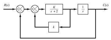
**Figure 5–75** Closed-loop system.
