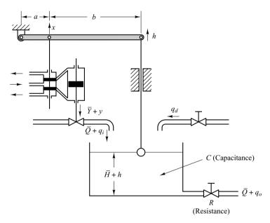
**Figure 4–52** Liquid-level control system.
