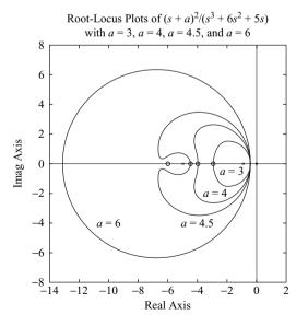
Figure 8–41 Root-locus plots of  $5K(s + a)^2/[s(s + 1)(s + 5)]$  when a = 3, a = 4, a = 4.5, and a = 6.
