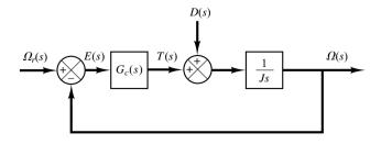
**Figure 5–69** Block diagram of a speed control system.
