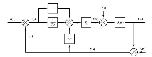
**Figure 8–26** PI-D-controlled system.
