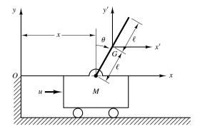
Figure 3–34 Inverted-pendulum system.
