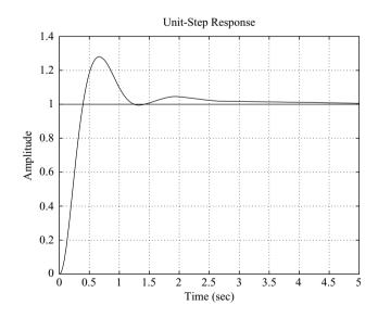
Figure 8–10 Unit-step response of the system shown in Figure 8–6 with PID controller having parameters  $K_p = 39.42$ ,  $T_i = 3.077$ , and  $T_d = 0.7692$ .
