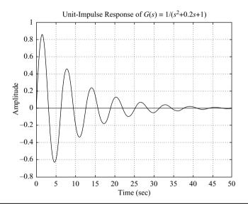
**Figure 5–24** Unit-impulse-response curve.
