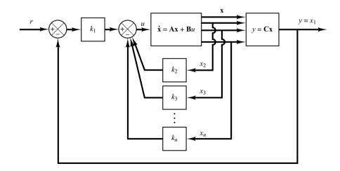
**Figure 10–4** Type 1 servo system when the plant has an integrator.
