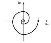
**Figure 7–32** Polar plot of  $e^{-j\omega L}/(1 + j\omega T)$ .
