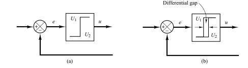
is called the *differential gap*. A differential gap is indicated in Figure 2–7(b). Such a differential gap causes the controller output u(t) to maintain its present value until the actuating error signal has moved slightly beyond the zero value. In some cases, the differential gap is a result of unintentional friction and lost motion; however, quite often it is intentionally provided in order to prevent too-frequent operation of the on–off mechanism.
