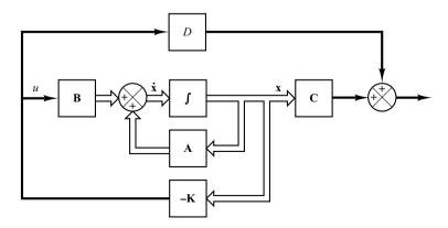
Figure 10–1 Closed-loop control system with  $u = -\mathbf{K}\mathbf{x}$ .
