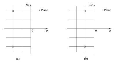
**Figure 7–64**Two systems with two closed-loop poles each.
