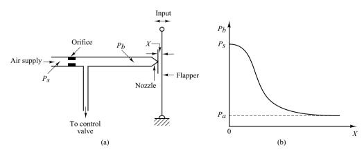
**Pneumatic Relays.** In practice, in a pneumatic controller, a nozzle–flapper amplifier acts as the first-stage amplifier and a pneumatic relay as the second-stage amplifier. The pneumatic relay is capable of handling a large quantity of airflow.
