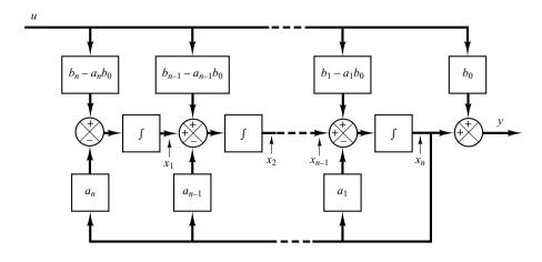
Figure 9–2 Block diagram representation of the system defined by Equations (9–78) and (9–79) (observable canonical form).
