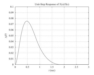
Figure 8–42 Response to unitstep disturbance input.
