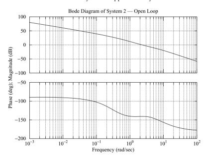
Figure 10–22 Bode diagram for the open-loop transfer function of System 2.
