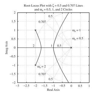
Figure 6–23 Constant  $\zeta$  lines and constant  $\omega_n$  circles superimposed on a root-locus plot.
