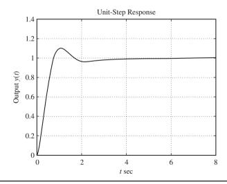
Figure 8–24 Unit-step response curve of the system with K = 3.2 and a = 0.9.
