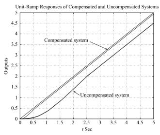
Figure 7–100 Unit-ramp response curves of the compensated and uncompensated systems.
