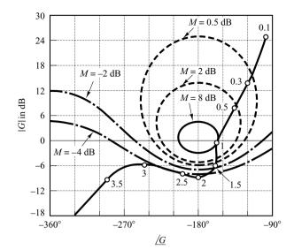
**Figure 7–142** Log-magnitude-versus-phase plot of G(s) given by Equation (7–32).
