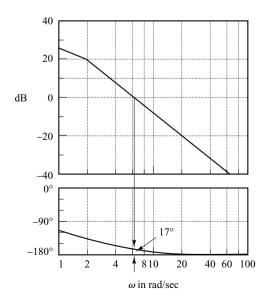
Figure 7-95 Bode diagram for  $G_1(j\omega) = 10G(j\omega)$ =  $40/[j\omega(j\omega + 2)]$
