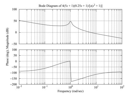
Figure 8–16 Bode diagram of  $4(5s + 1)(0.25s + 1)/[s(s^2 + 1)]$ .
