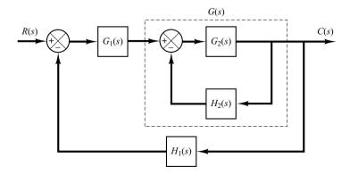
**Figure 7–59** Multiple-loop system.
