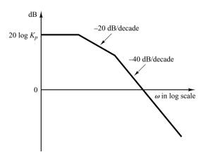
**Figure 7–17** Log-magnitude curve of a type 0 system.
