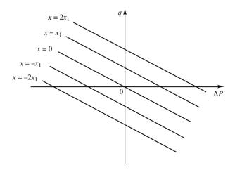
Figure 4–18 Characteristic curves of the linearized hydraulic servomotor.
