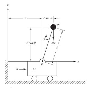
Figure 10–59 Inverted-pendulum system.
