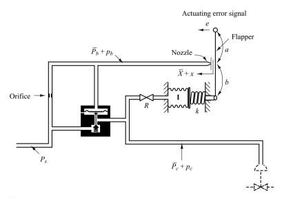
**Figure 4–46** Pneumatic controller.
