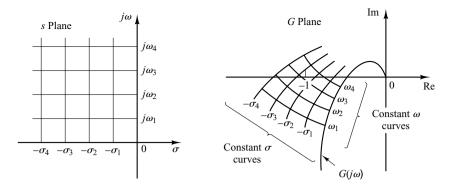
Figure 7–63 Conformal mapping of s-plane grids into the G(s) plane.
