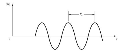
Figure 8–5 Sustained oscillation with period  $P_{cr}$ . ( $P_{cr}$  is measured in sec.)
