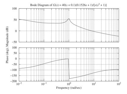
Figure 8–54 Bode diagram of G(s) = 40(s + 0.1) $(0.1526s + 1)/[s(s^2 + 1)].$
