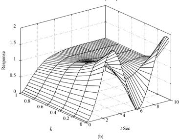
Figure 5–22 (a) Two-dimensional plot of unit-step response curves for  $\zeta = 0, 0.2, 0.4, 0.6, 0.8,$  and 1.0; (b) three-dimensional plot of unit-step response curves.
