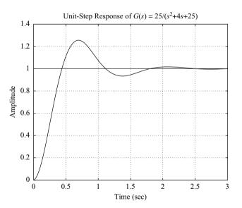
Figure 5–20 Unit-step response curve.
