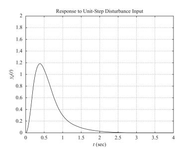
Figure 8–67 Response to unitstep disturbance input.
