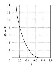
Figure 7–10  $M_r$ -versus- $\zeta$  curve for the second-order system  $1/[1 + 2\zeta(j\omega/\omega_n) + (j\omega/\omega_n)^2]$ .
