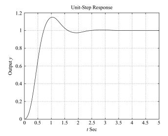
Figure 10–5 Unit-step response curve y(t) versus tfor the system designed in Example 10–4.
