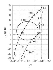
Figure 7–105 Log-magnitudeversus-phase plots of  $G_1$  (gain-adjusted but uncompensated open-loop transfer function) and  $G_cG$ (compensated openloop transfer function).
