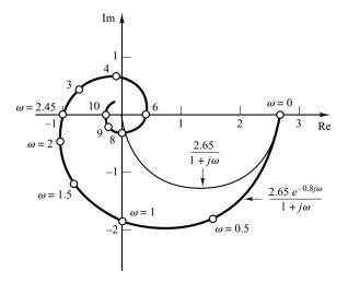
**Figure 7–126** Polar plots of  $2.65e^{-0.8j\omega}/(1+j\omega)$  and  $2.65/(1+j\omega)$ .
