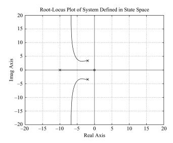
**Figure 6–20**Root-locus plot of system defined in state space, where **A**, **B**, **C**, and *D* are as given by Equation (6–15).
