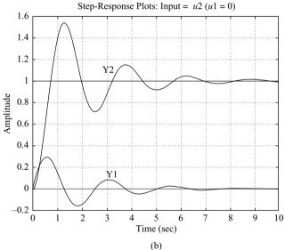
Figure 5–19 Unit-step response curves. (a)  $u_1$  is the input  $(u_2 = 0)$ ; (b)  $u_2$ is the input  $(u_1 = 0)$ .
