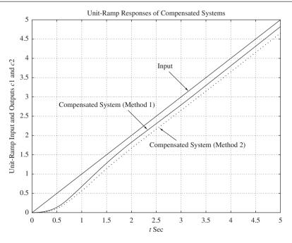
Figure 6–46 Unit-ramp response curves of designed systems.
