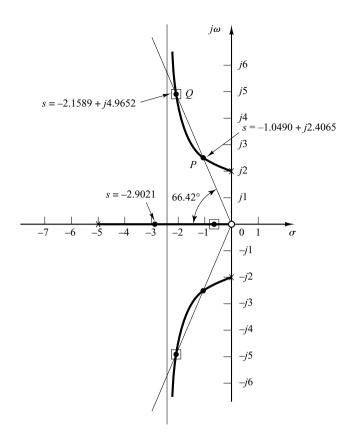
**Figure 6–62** Root-locus plot for the system shown in Figure 6–61.
