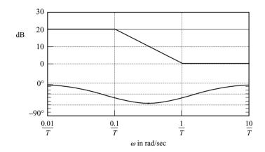
Figure 7–102 Bode diagram of a lag compensator  $\beta(j\omega T + 1)/(j\omega\beta T + 1)$ , with  $\beta = 10$ .
