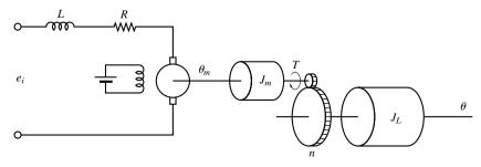
Figure 3–42 Armature-controlled dc servomotor system.
