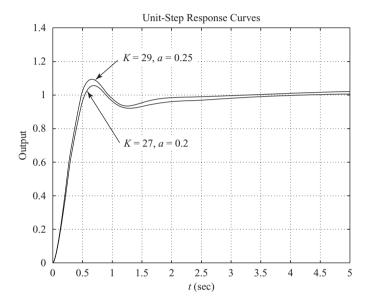
**Figure 8–65** Unit-step response curves.
