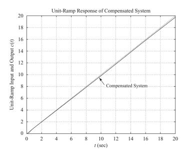
Figure 8–18 Unit-ramp input and the output curve.
