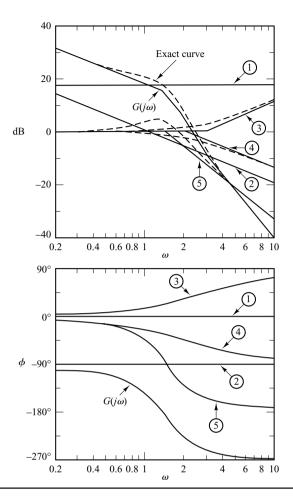
Figure 7–11 Bode diagram of the system considered in Example 7–3.
