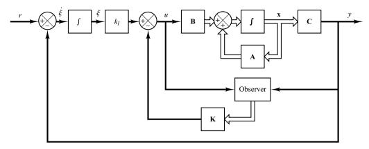
**Figure 10–7** Type 1 servo system with state observer.
