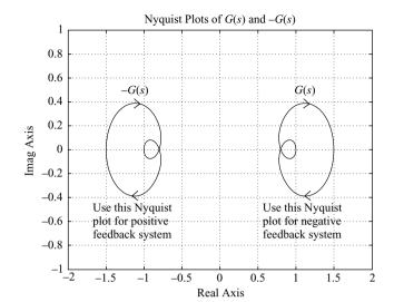
**Figure 7–131**Nyquist plots for positive-feedback system and negative-feedback system.
