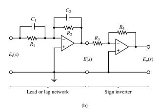
(a) Operational-amplifier circuit; (b) operational-amplifier circuit used as a lead or lag compensator.
