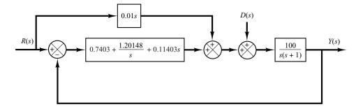
**Figure 8–69**Block diagram of the designed system.
