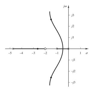
**Figure 6–43** Root-locus plot of the designed system.
