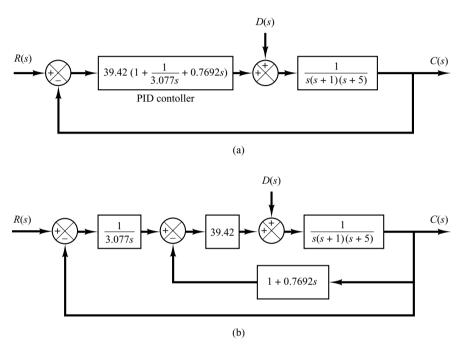
**Figure 8–73**(a) PID-controlled system; (b) I-PD-controlled system.
