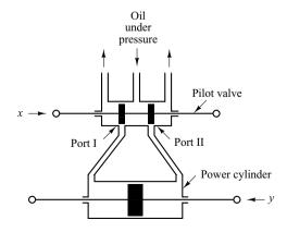
Figure 4–19 Hydraulic servomotor.
