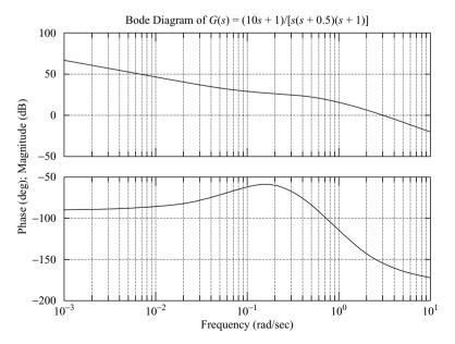
Figure 7–139 Bode diagram of  $G(s) = \frac{10s + 1}{s(s + 0.5)(s + 1)}.$
