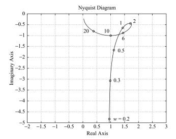
**Figure 7–129** Polar plot of  $G(j\omega)$  given in Problem **A–7–13**.
