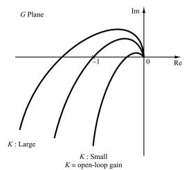
Figure 7-66 Polar plots of  $\frac{K(1 + j\omega T_a)(1 + j\omega T_b)\cdots}{(j\omega)(1 + j\omega T_1)(1 + j\omega T_2)\cdots}$
