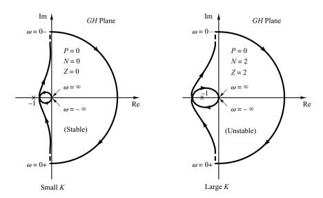
**Figure 7–54** Polar plots of the system considered in Example 7–15.
