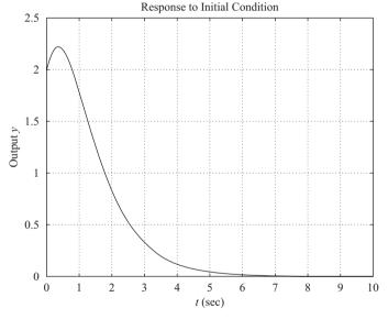
Figure 5–65 Response y(t) to the given initial condition.
