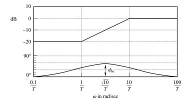
Figure 7–92 Bode diagram of a lead compensator  $\alpha(j\omega T + 1)/(j\omega\alpha T + 1)$ , where  $\alpha = 0.1$ .
