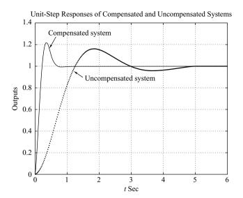
Figure 7–99 Unit-step response curves of the compensated and uncompensated systems.
