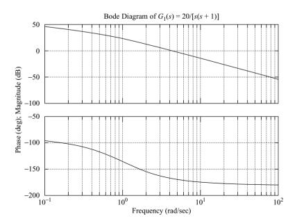
**Figure 7–145** Bode diagram of  $G_1(s)$ .
