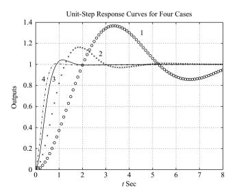
Figure 5–59 Unit-step response curves for four cases.
