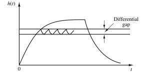
Figure 2–9 Level h(t)-versus-t curve for the system shown in Figure 2–8(a).
