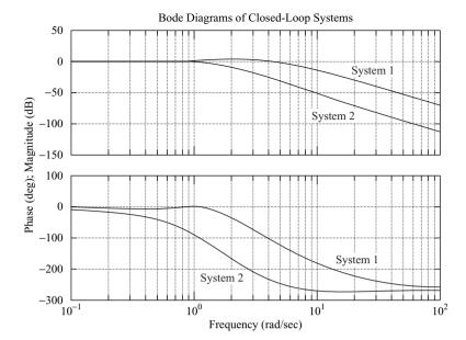
Figure 10–34 Bode diagrams of closed-loop system 1 (shown in Figure 10–29) and closedloop system 2 (shown in Figure 10–31).
