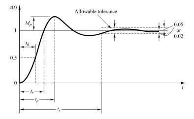
Figure 5–8 Unit-step response curve showing  $t_d$ ,  $t_r$ ,  $t_p$ ,  $M_p$ , and  $t_s$ .
