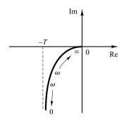
Figure 7–31 Polar plot of  $1/[j\omega(1+j\omega T)]$ .
