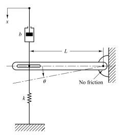
**Figure 5–49** Mechanical system.
