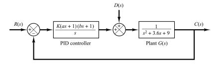
Figure 8–47 PID-controlled system.
