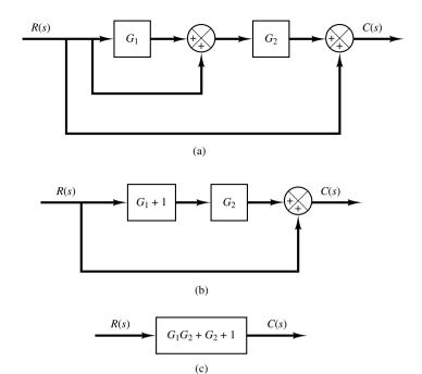
Figure 2–20 Reduction of the block diagram shown in Figure 2–19.
