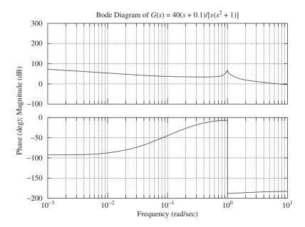
Figure 8–53 Bode diagram of  $G(s) = \frac{40(s + 0.1)}{[s(s^2 + 1)]}$ .
