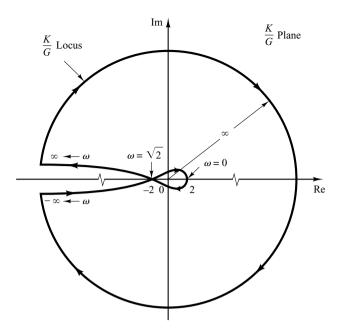
**Figure 7–132** Polar plot of  $K/G(j\omega)$ .
