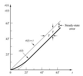
Figure 5–3 Unit-ramp response of the system shown in Figure 5–1(a).
