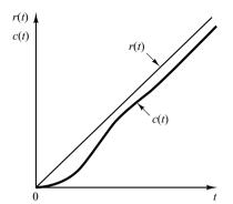
Figure 5–47 Response of a type 1 unity-feedback system to a ramp input.
