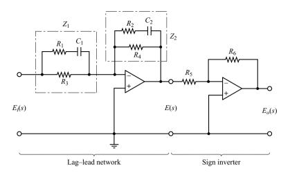
**Figure 6–53** Lag–lead compensator.
