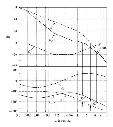
Figure 7–111 Bode diagrams for G (gain-adjusted but uncompensated open-loop transfer function),  $G_c$  (compensator), and  $G_cG$  (compensated open-loop transfer function).
