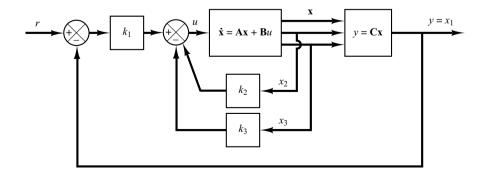
**Figure 10–58** Type 1 servo system.
