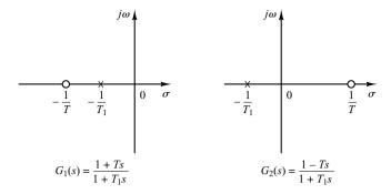
Figure 7–12 Pole–zero configurations of a minimum-phase system  $G_1(s)$  and nonminimum-phase system  $G_2(s)$ .
