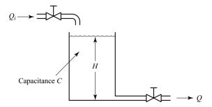
**Figure 4–27** Liquid-level system.
