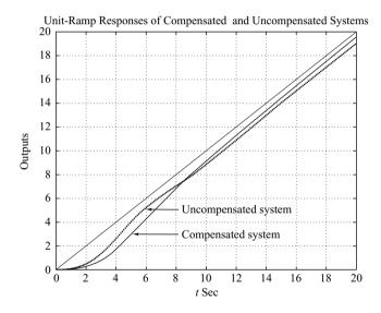
Figure 7–107 Unit-ramp response curves for the compensated and uncompensated systems (Example 7–27).
