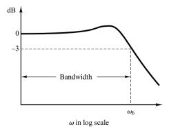
Figure 7–76 Plot of a closed-loop frequency response curve showing cutoff frequency  $\omega_b$  and bandwidth.
