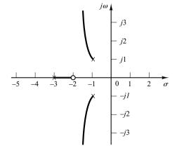
Figure 6-32 Root-locus plot for the negative-feedback system with  $G(s) = K(s+2)/[(s+3)(s^2+2s+2)],$
