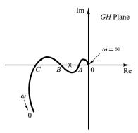
**Figure 7–58**Polar plot of a conditionally stable system.
