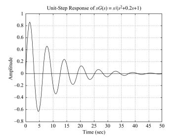
Figure 5–25 Unit-impulseresponse curve obtained as the unitstep response of  $sG(s) = s/(s^2 + 0.2s + 1)$ .
