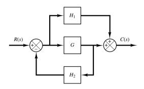
**Figure 2–17** Block diagram of a system.
