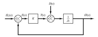
Figure 5–67 Block diagram of a speed control system.
